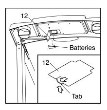
two batteries into the console. Make sure that the negative (–) ends of the batteries are touching the springs. Close the battery cover, push up on the tab, and then push the tab forward as shown in the inset drawing. Make sure that the tab locks into place.
